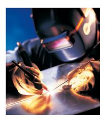
Welding technique for ferritic stainless steels needs to be 'finetuned' by welders used to austenitic stainless grades.
